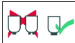
Use the correct crucible stand which must be central and support the whole base.
