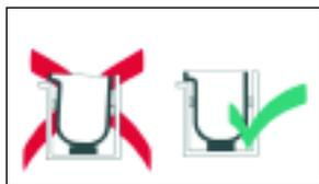
Use correctly positioned grip bricks in tilting furnaces, leaving gaps for expansion. Do not hang crucible on spout.
